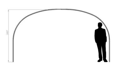
The hoops in this model are heavy gauge high tensile steel as standard and have a new coating that is 20 times more corrosion resistant than galvanised steel. 8 brace bars are supplied.
